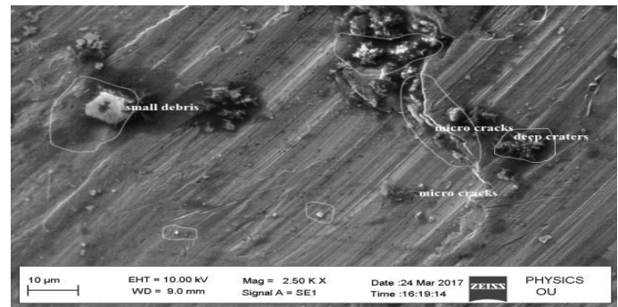
Fig 6.2 Micro structure of the machined sample at experiment no 1, low surface finish
